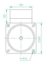
Motor, Gearbox with Lead Wires
